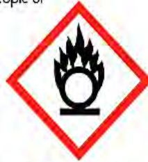
May cause fire or enhance the combustion of other materials
